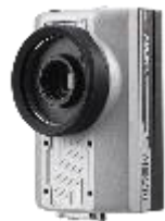
NEON-2000-JT2 Series NVIDIA® Jetson™ TX2-based
